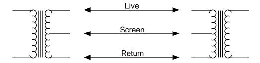
The coils of the transformer are wired anti phase! 1 clockwise, the other anti clockwise. This cancels out any hum pickup.in the cable length.
