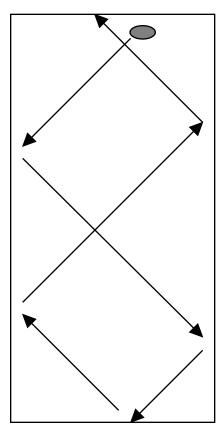
Sound 'bounces' around inside a building. The size, shape, and construction of the walls all play a part on the way sound behaves.
