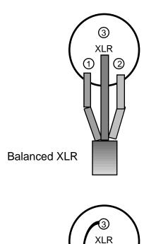
For unbalanced connection: Pins 1 & 3 are wired together.
